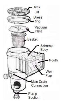
The skimmer box has a weir door at the front. The weir door floats vertically when the pump is off, preventing leaves and debris from going back into the pool. When the pump and filter is operating, the weir door acts as a floating skimmer to draw dirt, leaves and other waste into the skimmer box.
